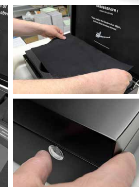
Fitting the watch holder and the cover plate
